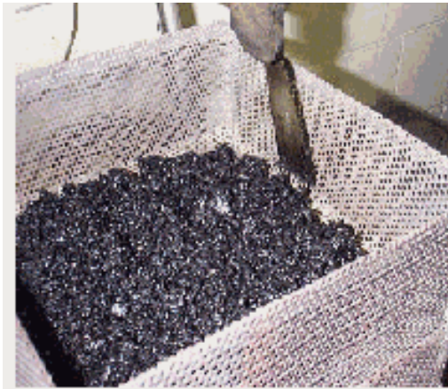
Asphalt Placed in Basket
